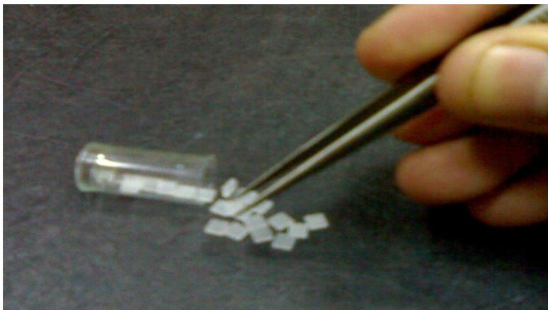
**Fig. (4) Handling and preparation of Chips Dosimeter TLD-100**
