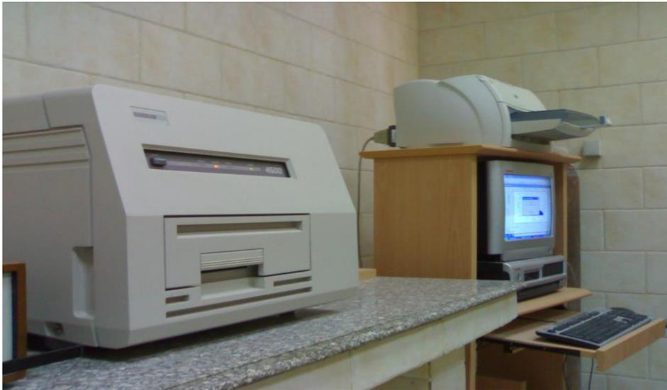
**Fig. (3) The Harshaw TLD reader**
