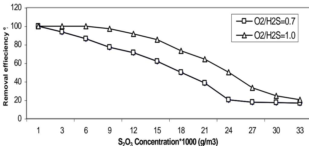
Figure(7): Effect of Thiosulfate( $S_2O_3^{2-}$ ) concentration on  $H_2S$  bioremediation
