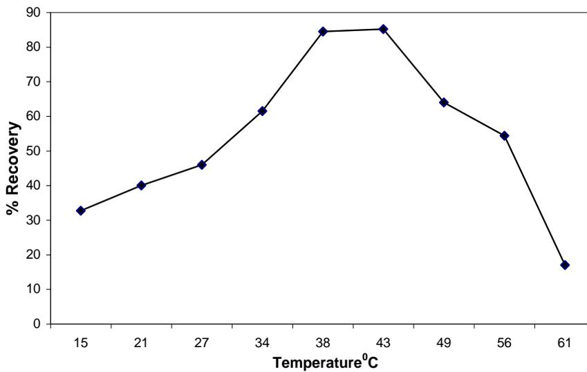
Figure(3): Effects of temperature on H<sub>2</sub>S bioremediation
