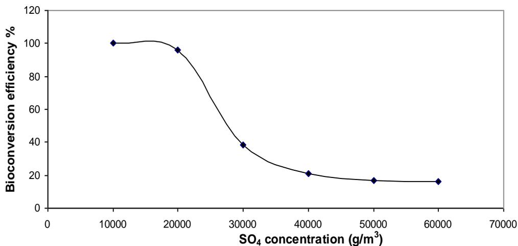
**Figure(6): effect of SO<sub>4</sub> concentration on H<sub>2</sub>S bioremediation**
