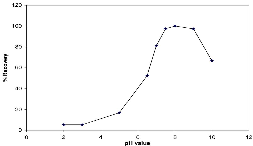
Figure (4) : effects of pH on H<sub>2</sub>S bioremediation
