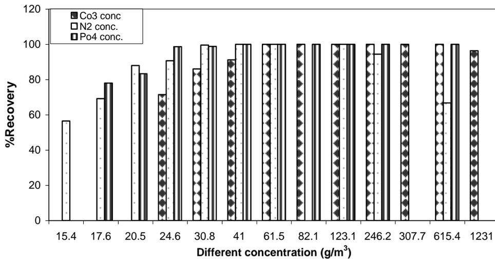
Figure (2): Effects of different concentration of nutrients on H<sub>2</sub>S bioremediation
